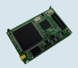
The Nano Series features robust, high speed, low latency, secure data communications. The n3420 has full serial and diagnostics data capabilities. The n3420 offers excellent noise figure, superior interference rejection, agile frequency synthesis, digital modulation, and matched filter detection.
